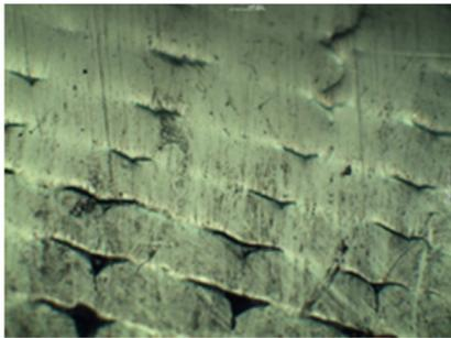
(a) Fracture after cooling in the refrigerator
