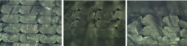
(b) Optical micrograph ( $\times 100$ ) of the specimen fabricated at 245 °C, 260 °C, and 275 °C from left to right
