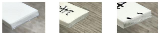
(a) Simple fracture (b) Fracture after cooling in the refrigerator (c) Fracture after cooling using dry ice
