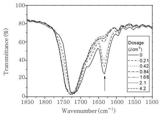
**Figure 3.** Partial IR spectra of the MIP system showing a reaction-induced peak change at  $1635\text{ cm}^{-1}$ .
