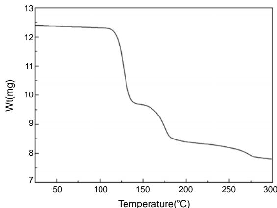
**Figure 1.** TGA thermogram of a chemical blowing agent used in this study.
