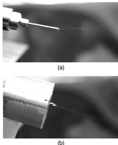
**Figure 3.** Photographs taken with a digital camera: (a) unstable initial spun jets of normal electrospinning and (b) stable initial spun jets by using an auxiliary cylindrical electrode under the applied same electric voltage.
