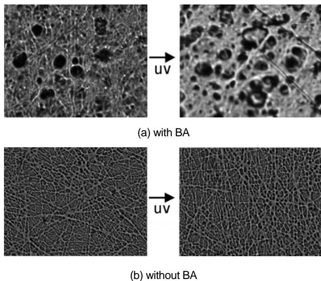
**Figure 9.** Pore-structure change under the UV exposure of PCL nanofiber mats: (a) with and (b) without a blowing agent.
