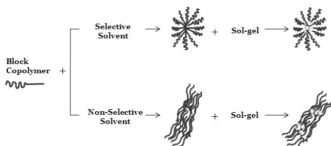
**Figure 1.** Schematic representation of the self-assembly of block copolymer in solution with different solvent selectivity.
