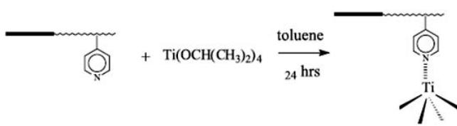
**Figure 3.** Schematic diagram of the complex formation between titanium isopropoxide and the PS-P4VP micelle core.
