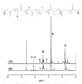
**Figure 2.** <sup>1</sup>H NMR spectra of PLGA-PEG-PLGA triblock copolymer (a); PLGA-PEG-PLGA diacrylate (b).
