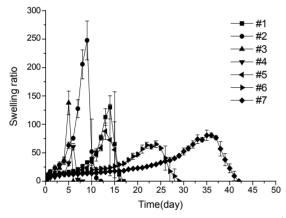
**Figure 3.** *In vitro* degradation test of PLGA-PEG-PLGA/PEG hydrogels at 37 °C.
