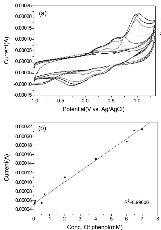
**Figure 5.** Cyclic voltammograms of the EMB in a 0.1 M phosphate buffer solution ( $\text{pH}=7.0$ ) containing different phenol concentration (a) (from a to j: 0, 0.05, 0.1, 0.5, 0.7, 2, 4, 6, 6.5, 7.0 mM) with a scan rate of 100 mV/s and calibration plot of the concentration of phenol with respect to the current (b).
