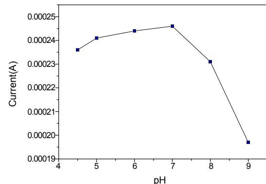
**Figure 6.** Effect of pH on the response of the EMB in a 0.1 M phosphate buffer solution ( $\text{pH}=4.5, 5, 6, 7, 8$ , and 9) containing 5 mM phenol at a scan rate of 100 mV/s.
