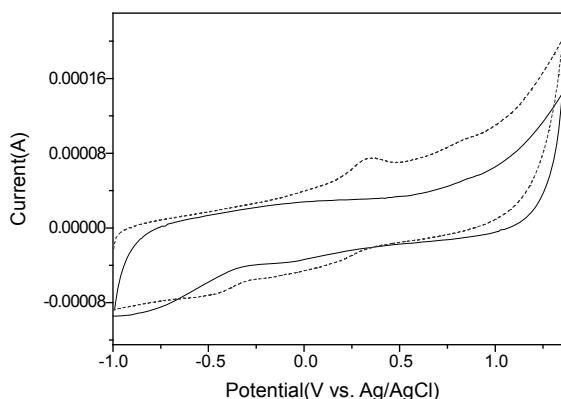
**Figure 7.** Cyclic voltammograms of the EMB in a 0.1 M phosphate buffer solution (solid line) containing 100  $\mu\text{L}$  of red wine (AMOR) (dashed line) with a scan rate of 100 mV/s.
