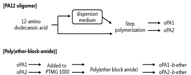
**Figure 3.** Reaction flow of PA12 oligomers and PEBA.
