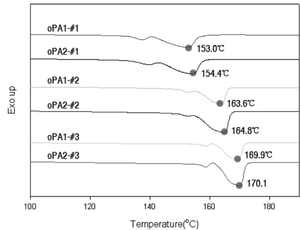
**Figure 6. DSC thermograms of oPA1 and oPA2.**
