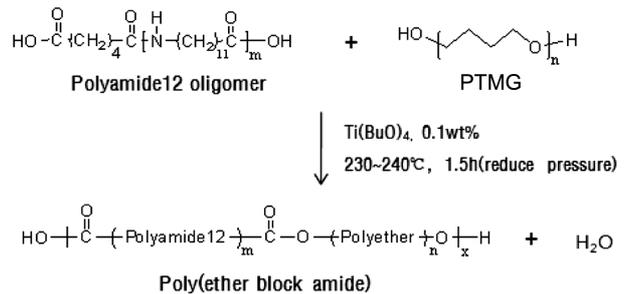
**Figure 2.** Reaction scheme of step polymerization for PEBA.
