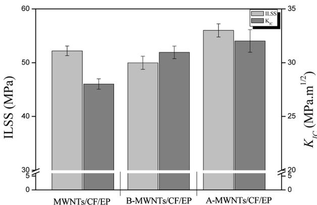
Figure 3. ILSS and  $K_{IC}$  results of the composites.
