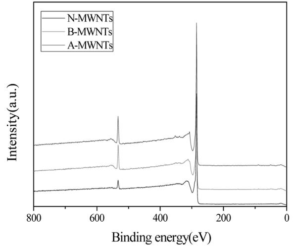
Figure 2. XPS survey of chemically modified MWNTs.
