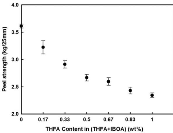
Figure 3. Peel strengths of PSAs with THFA content.
