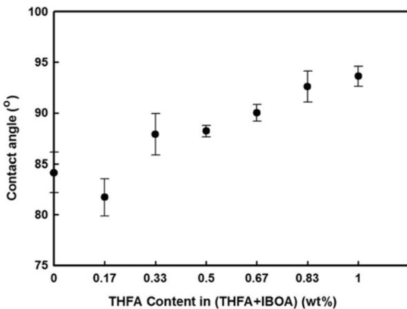
Figure 4. Contact angles of the PSAs with THFA content.
