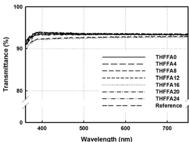
Figure 6. Transmittances of the PSAs with THFA content.
