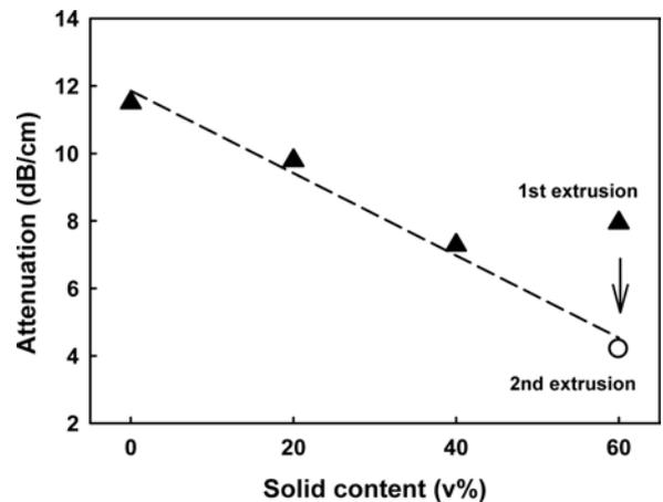
Figure 11. Ultrasonic attenuation vs. solid content for EVA31/Dechlorane suspensions.
