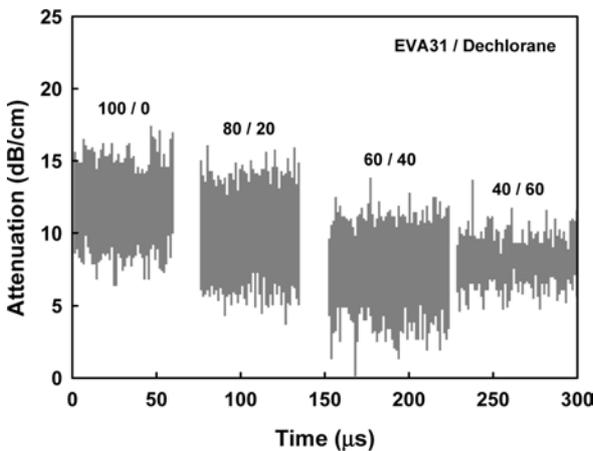
Figure 9. Attenuation of EVA31/Dechlorane suspensions at 120°C.
