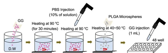
Figure 2. Fabrication process of the gellan gum scaffolds containing PLGA microspheres.
