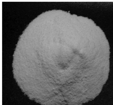
**Figure 1.** Appearance of the dry s-PLA powder.
