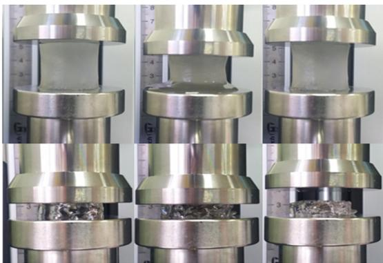
**Figure 2.** Compression test on PASP-cryogel (a, at strain 30%); conventional gel (b, at strain 18%).
