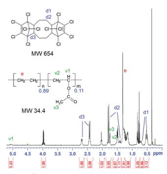
Figure 10. <sup>1</sup>H NMR spectra of PBX simulant in benzene-d.
