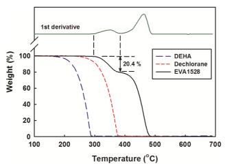
**Figure 2.** TGA thermograms of neat DEHA, Dechlorane, and EVA, and DTG thermogram of EVA.
