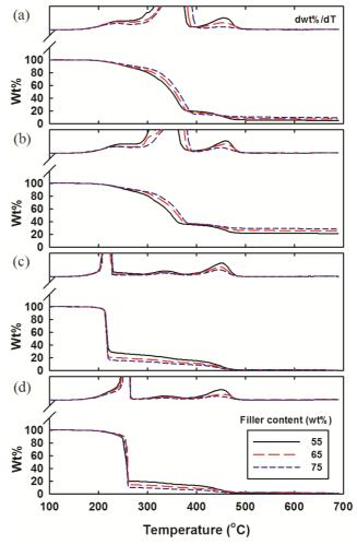
**Figure 3.** TGA and DTG thermograms of PBX and PBX simulant with various fillers: (a) Dechlorane; (b) Dechlorane/aluminum; (c) RDX; (d) HMX.
