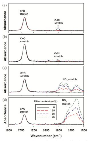
**Figure 6.** ATR spectra of PBX and PBX simulant with various fillers: (a) Dechlorane; (b) Dechlorane/aluminum; (c) RDX; (d) HMX.
