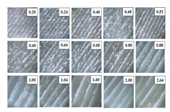
**Figure 7.** Optical micrograph of CO<sub>2</sub> laser sintered samples as a function of energy density.
