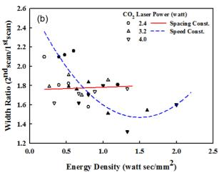
**Figure 4.** Effect of  $CO_2$  laser scan spacing and scan speed on: (a) the single width of sintered sample; (b) width ratio between  $1^{st}$  scan and  $2^{nd}$  scan (open symbol with solid line; constant scan spacing, closed symbol with broken line; constant scan speed).
