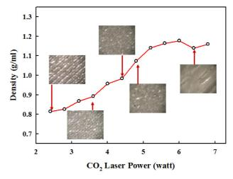
**Figure 5.** Effect of CO<sub>2</sub> laser power on the density of sintered samples with different surface morphology.
