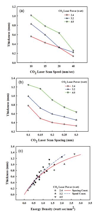
**Figure 3.** Effect of CO<sub>2</sub> laser scan spacing and scan speed on the thickness of sintered sample: (a) scan spacing; (b) scan speed; (c) energy density (open symbol with solid line; constant scan spacing, closed symbol with broken line; constant scan speed).
