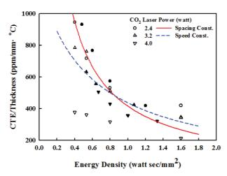
**Figure 9.** Effect of laser scan speed and scan spacing on the coefficient of thermal expansion of sintered sample (open symbol with solid line; constant scan spacing, closed symbol with broken line; constant scan speed).
