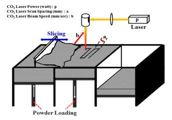
**Figure 1.** Schematics of SLS 3D printer used in this study (p; laser power a: laser scan spacing, b: laser scan speed).
