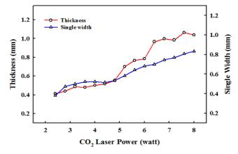
Figure 2. Effect of CO<sub>2</sub> laser power on the shaping dimension of sintered samples.
