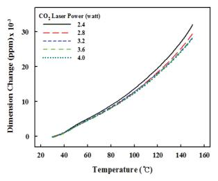
Figure 8. TMA thermogram of sintered samples by CO<sub>2</sub> laser.
