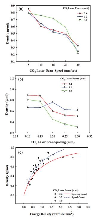
**Figure 6.** Effect of CO<sub>2</sub> laser scan spacing and scan speed on the density of sintered sample: (a) scan spacing; (b) scan speed; (c) energy density (open symbol with solid line; constant scan spacing, closed symbol with broken line; constant scan speed).
