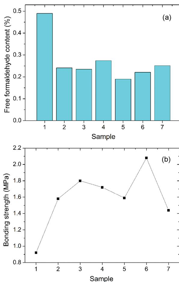
**Figure 4.** Free formaldehyde content (a); bonding strength (b) of sample 1 ~ sample 7.
