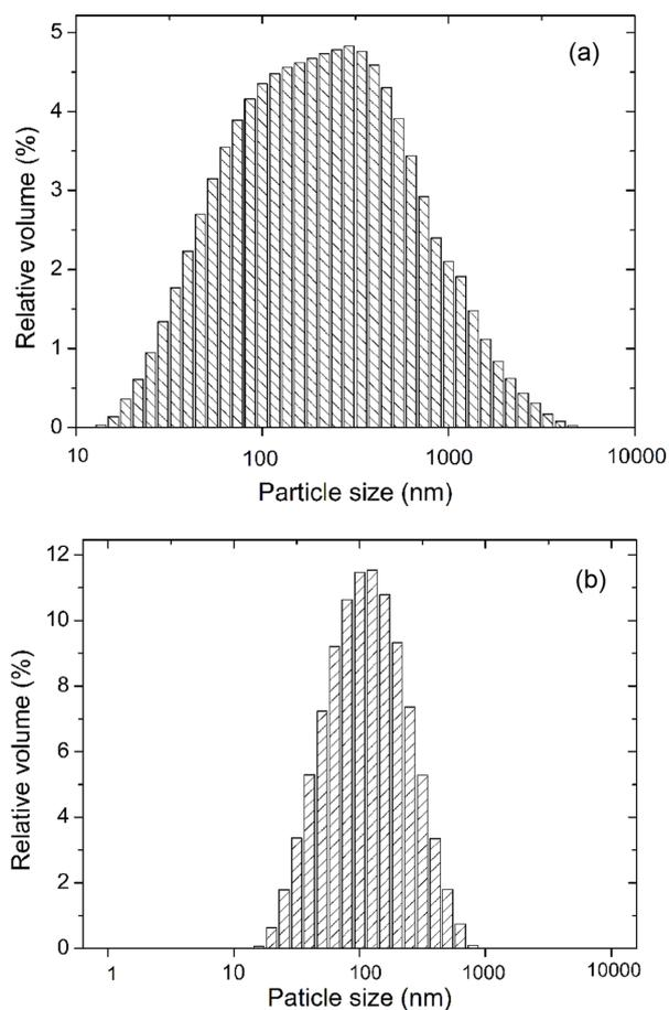
**Figure 1.** Particle size of pure (a); modified (b) nano-SiO<sub>2</sub>.
