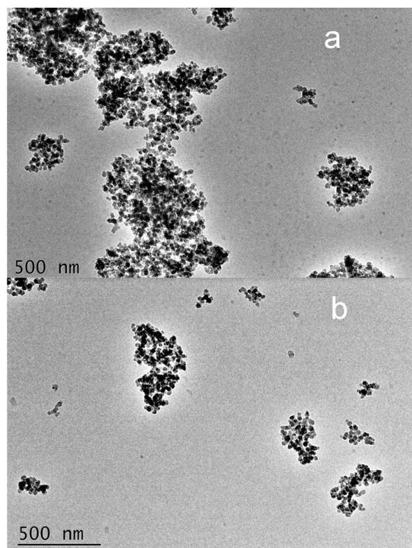
**Figure 2.** TEM microphotographs of pure nano-SiO<sub>2</sub> (a); modified nano-SiO<sub>2</sub> (b).
