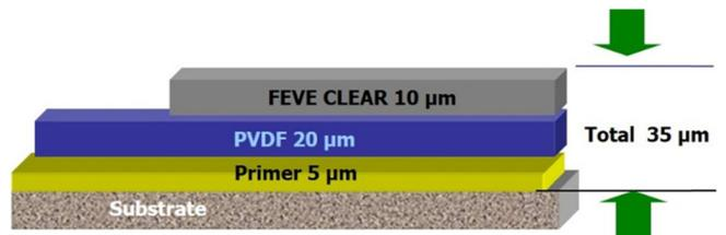
Figure 4. Schematic layer structure of coating system.
