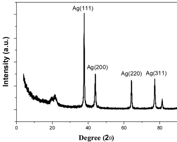
**Figure 7.** XRD patterns of cotton fibers coated with silver nanoparticles.
