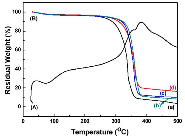
**Figure 10.** (A) DSC; (B) TGA analysis of cotton/Ag fibers with different silver content fibers.
