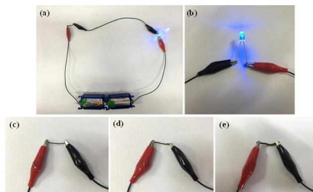
**Figure 12.** Conductive silver coated cotton fibers ties into a simple circuit: (a) knotting one end to a battery and the other to an LED; (b) lighted LED lamp and tied with (c) 10-ply; (d) 20-ply and (e) 30-ply of AgNPs-coated cotton fiber.
