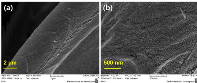
**Figure 8.** SEM images of washed silvered cotton fiber at magnification (a) 20 kx; (b) 100 kx.
