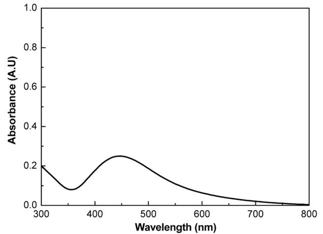
**Figure 9.** UV-visible spectrum of AgNPs-dispersed colloidal solution obtained after washing of cotton fiber/AgNPs.
