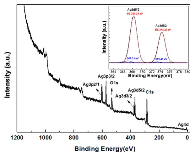
**Figure 5.** XPS spectra of Ag coated cotton fiber. Inset figure: deconvoluted Ag3d XPS spectra of cotton fiber surface.
