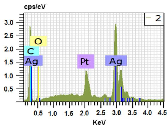
**Figure 6.** EDX analysis patterns of Ag coated cotton fiber treated with 5% silver carbamate complex.
