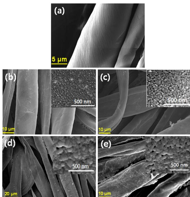
**Figure 4.** SEM images of (a) pristine cotton fiber; (b) cotton/Ag(2%); (c) cotton/Ag(5%); (d) cotton/Ag(7%); (e) cotton/Ag(10%); inset figure was captured with a magnification setting of 100 kx.
