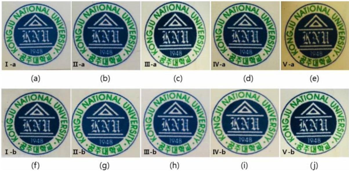
**Figure 4.** Photographs of colorless polyimide with varying concentrations of the anhydride and diamine: (a)-(e) sulfone based TPI; (f)-(j) sulfone-siloxane based TPI.
