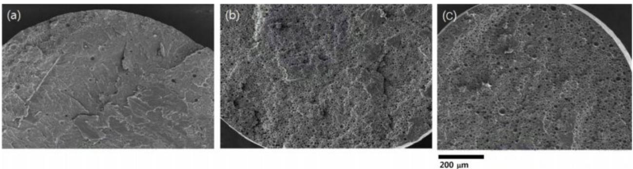
Figure 7. SEM images of WEPS beads at 300× magnification: (a) Styrene : emulsified water = 9:1; (b) styrene : emulsified water = 8:2; (c) styrene : emulsified water = 7:3.
