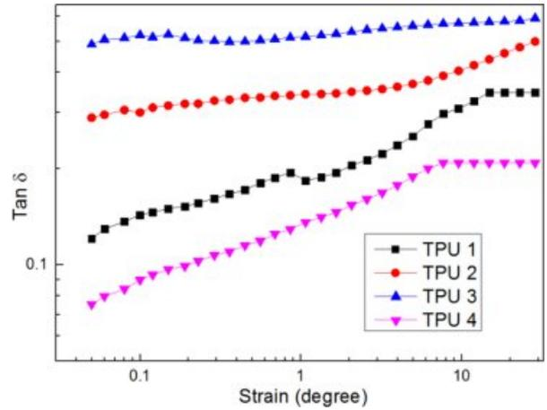
Figure 7. Loss factor of TPU samples.
