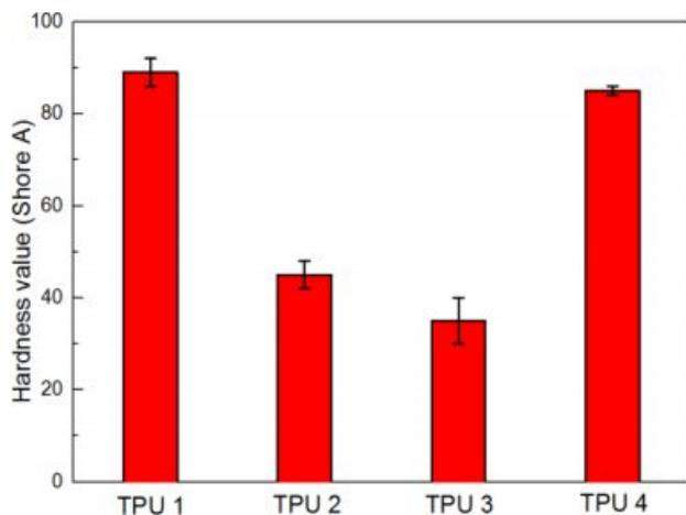
**Figure 10.** Hardness of TPU samples.
