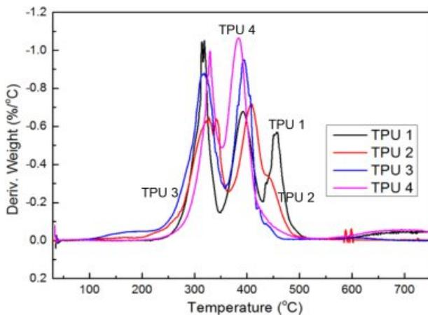
**Figure 2.** Derivative of weight according to temperature changes of TPU samples.
