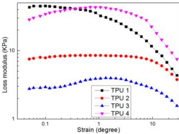
Figure 6. Loss modulus of TPU samples.
