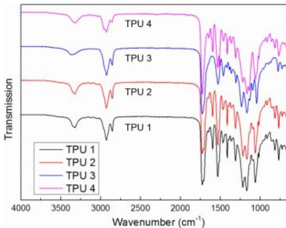
**Figure 3.** FTIR spectra of TPU samples.
