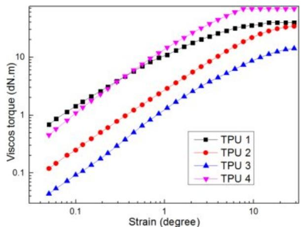
Figure 9. Viscous torque of TPU samples.
