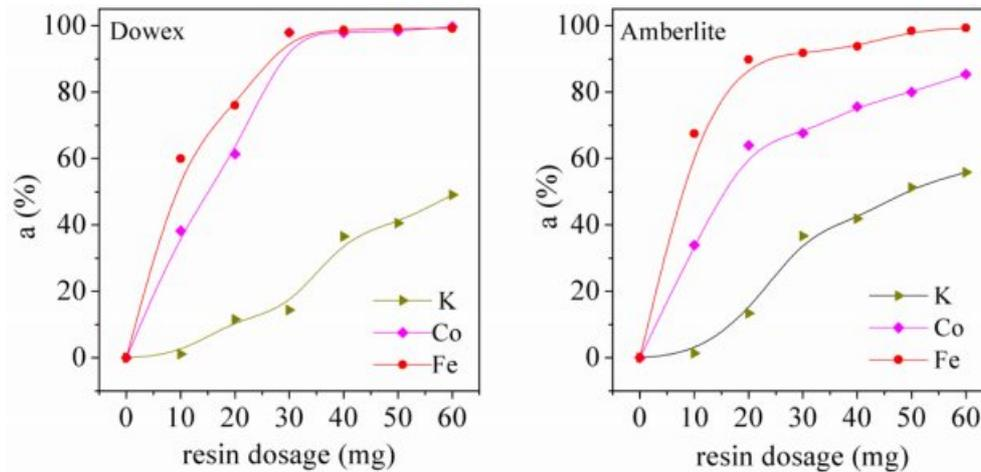
**Figure 10.** Selective adsorption ratio of Fe(III), Co(II), K(I) in 321-MMS.
