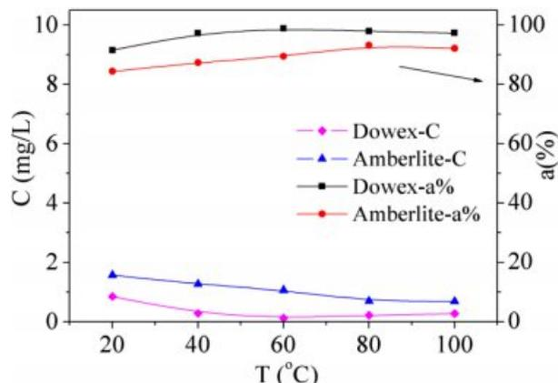
**Figure 2.** Effect of temperature on adsorption of Fe(III) (iron concentration = 10 mg/L, 20 mg/100 mL, pH = 2, 100 min).
