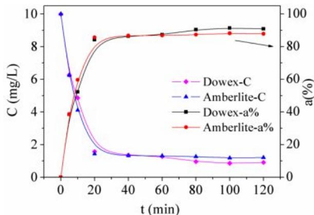
**Figure 1.** Effect of contact time on adsorption of Fe(III) (iron concentration = 10 mg/L, 25 °C, 20 mg/100 mL, pH = 2).
