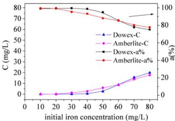
**Figure 5.** Effect of iron concentration on adsorption of Fe(III) (50 mg/100 mL, 100 min, pH = 3, 60 °C for Dowex resin, 80 °C for Amberlite resin).
