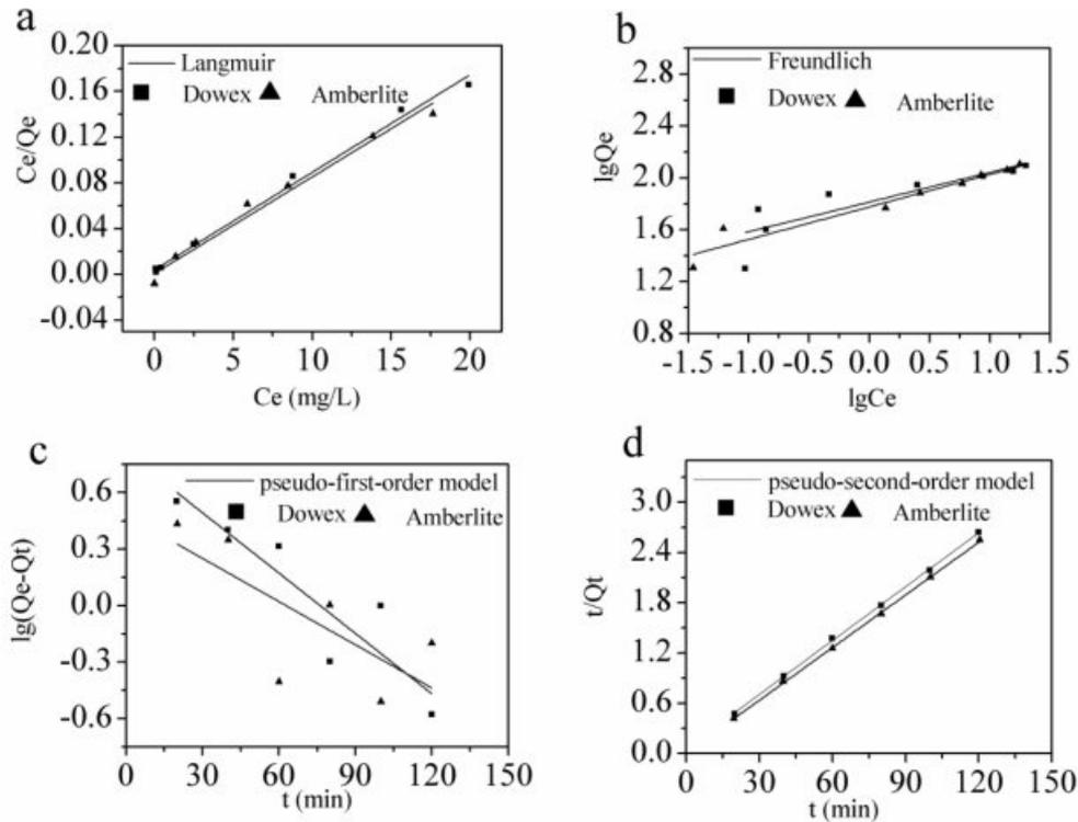
**Figure 7.** Adsorption model (Langmuir-a, Freundlich-b); The kinetics (pseudo-first-order model-c, pseudo-second-order model-d) for Fe(III) adsorption.
