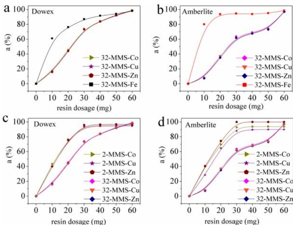
**Figure 9.** Comparison of adsorption ratios of Fe(III), Co(II), Cu(II), Zn(II) in multi-metal systems.
