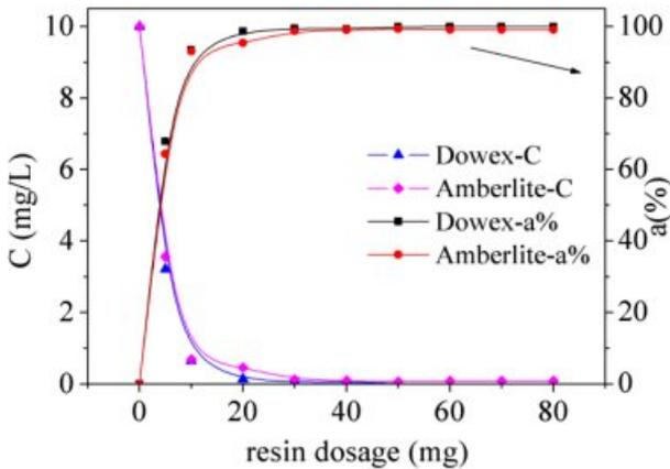
**Figure 4.** Effect of resin dosage on adsorption of Fe(III) (iron concentration = 10 mg/L, 100 min, pH = 3, 60 °C for Dowex resin, 80 °C for Amberlite resin).
