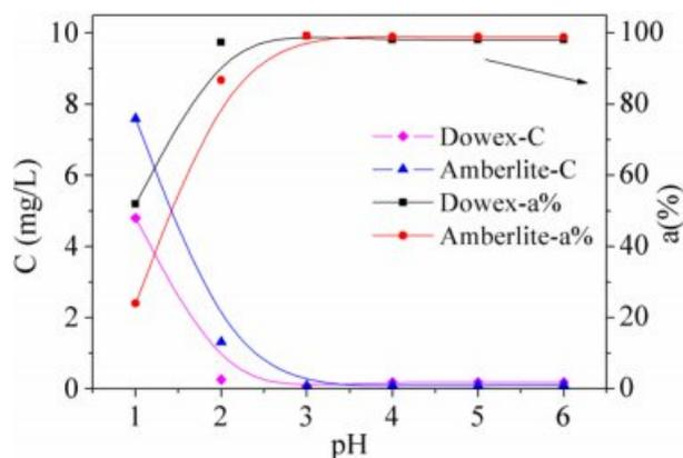
**Figure 3.** Effect of pH on adsorption of Fe(III) (iron concentration = 10 mg/L, 20 mg/100 mL, 100 min, 60 °C for Dowex resin, 80 °C for Amberlite resin).
