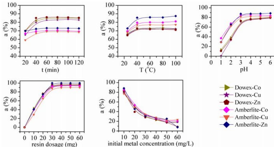
**Figure 8.** Adsorption ratio of Co(II), Cu(II), Zn(II) with different contact time, temperature, pH, resin dosage and initial concentration in 2-MMS.
