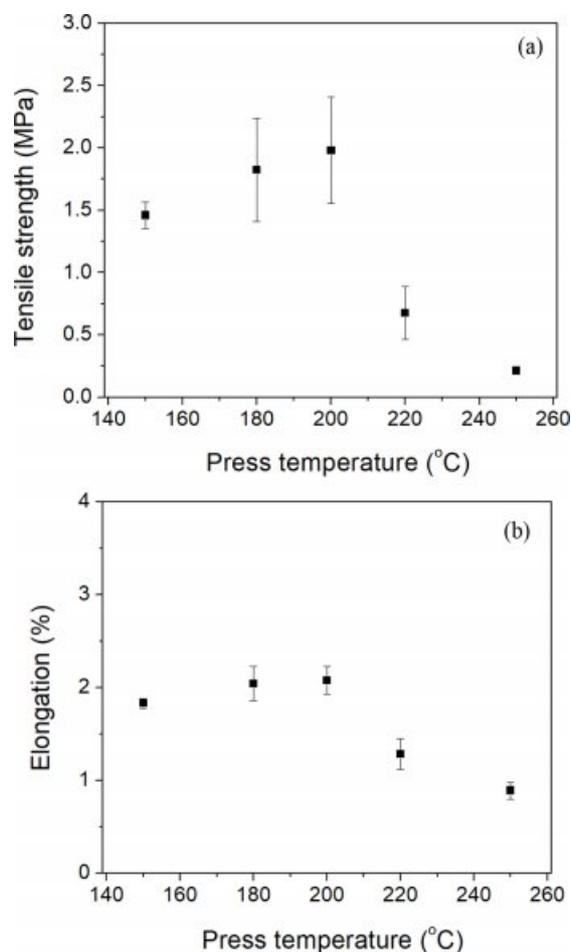
**Figure 6.** Mechanical properties of the airlaid nonwoven silk fabric prepared with different press temperatures: (a) tensile strength; (b) elongation.
