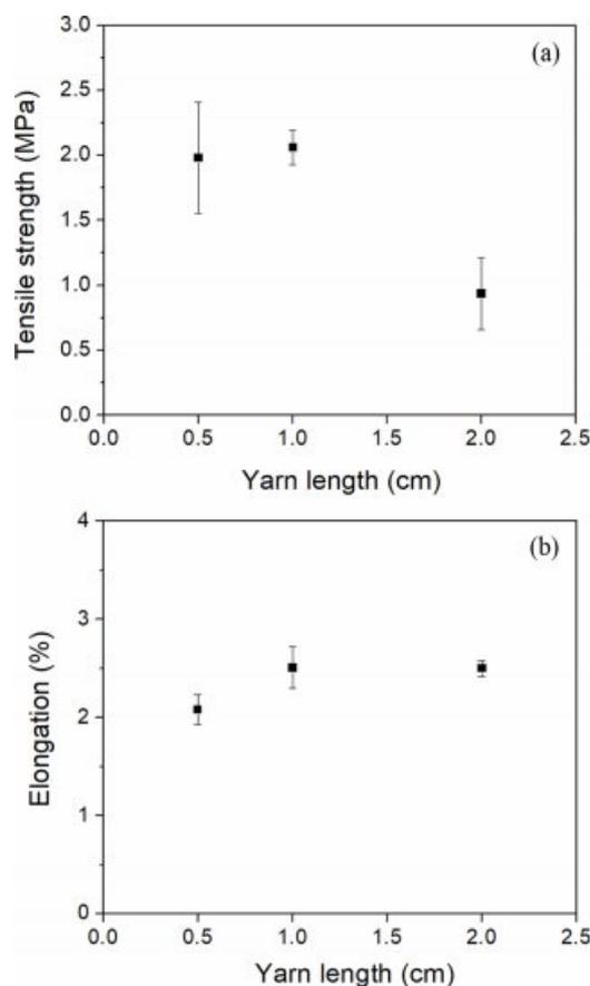
**Figure 3.** Mechanical properties of the airlaid nonwoven silk fabric with different yarn lengths: (a) tensile strength; (b) elongation.
