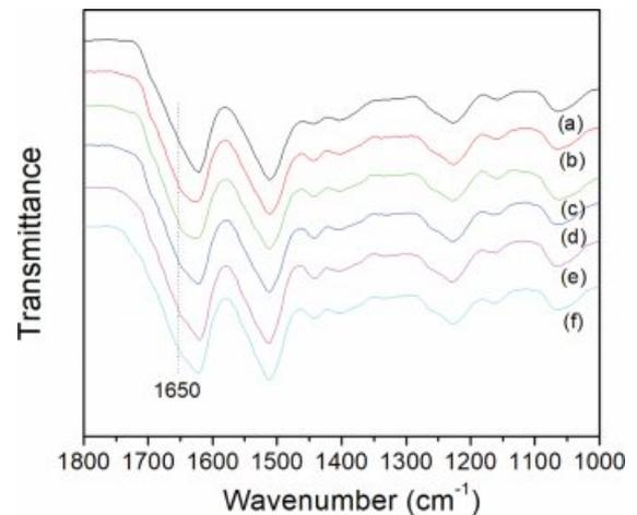
**Figure 5.** FTIR spectra of airlaid nonwoven silk fabric prepared at different press temperatures: (a) untreated; (b) 150 °C; (c) 180 °C; (d) 200 °C; (e) 220 °C; (f) 250 °C.
