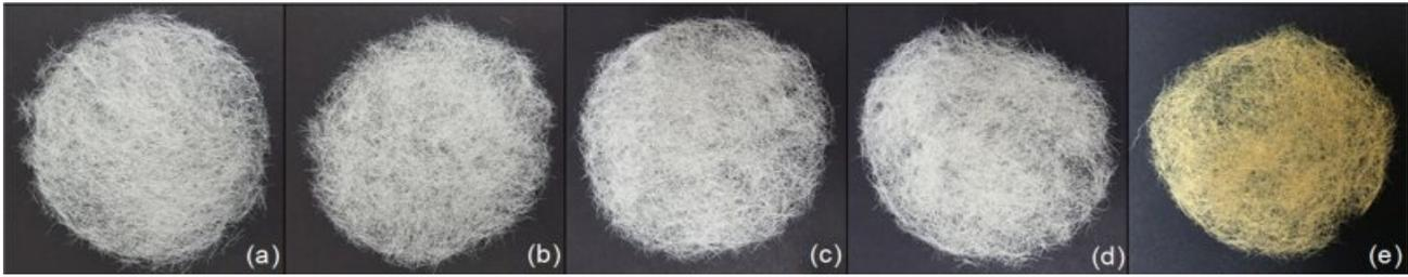
**Figure 4.** Airlaid nonwoven silk fabric prepared at different press temperatures: (a) 150 °C; (b) 180 °C; (c) 200 °C; (d) 220 °C; (e) 250 °C.
