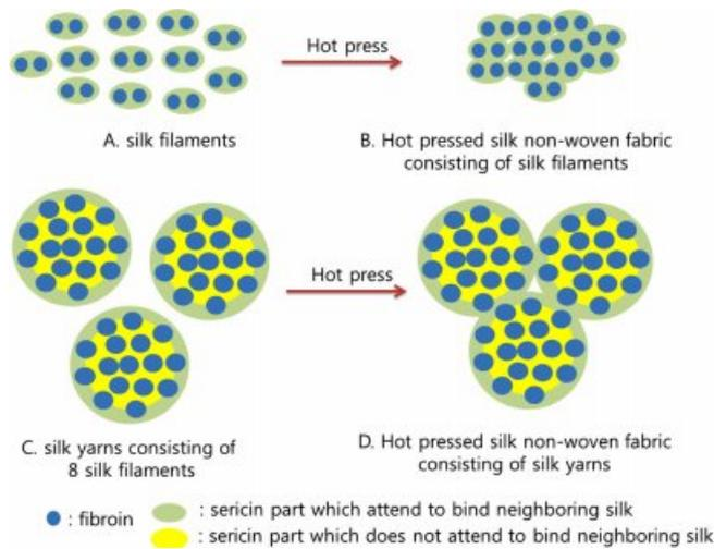
**Figure 7.** Difference in the binding of sericin in silk filament and silk yarn.
