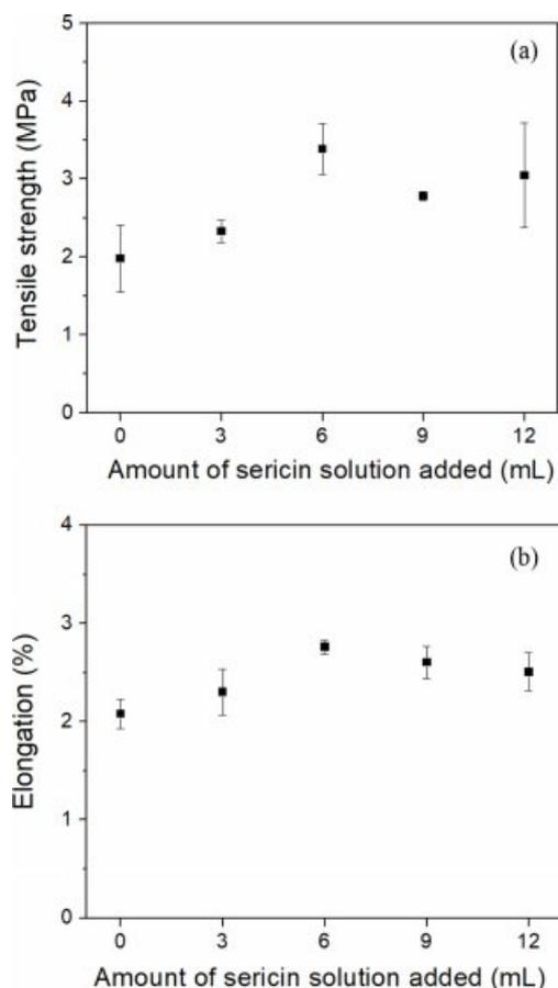
**Figure 10.** Mechanical properties of the airlaid nonwoven silk fabric prepared with different amounts of 2.5% (w/w) aqueous sericin solution: (a) tensile strength; (b) elongation.
