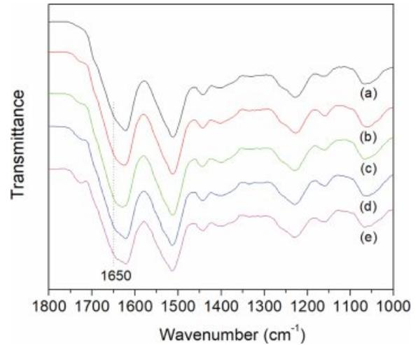
**Figure 9.** FTIR spectra of airlaid nonwoven silk fabric prepared with different amounts of 2.5% (w/w) aqueous sericin solution: (a) 0 mL; (b) 3 mL; (c) 6 mL; (d) 9 mL; (e) 12 mL.
