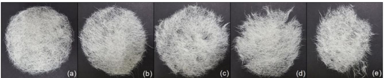
**Figure 8.** Airlaid nonwoven silk fabric prepared with different amounts of 2.5% (w/w) aqueous sericin solution: (a) 0 mL; (b) 3 mL; (c) 6 mL; (d) 9 mL; (e) 12 mL.
