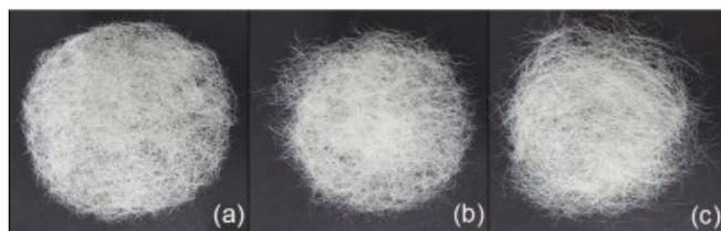
**Figure 2.** Airlaid nonwoven silk fabric with different yarn lengths: (a) 0.5 cm; (b) 1 cm; (c) 2 cm.
