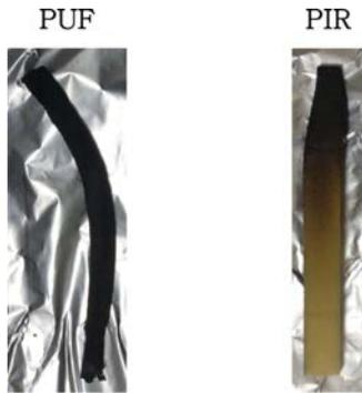
**Figure 6.** PUF and PIR foam after UL-94 vertical burning test (HFO-1233zd).
