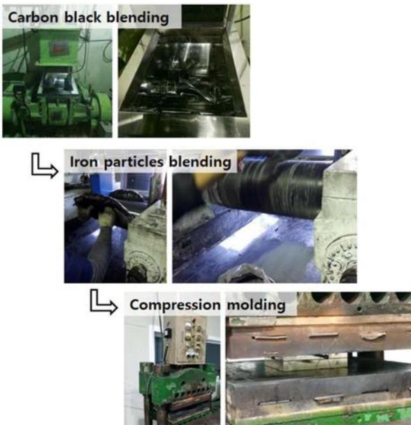
Figure 2. Fabrication process of MRE specimens.
