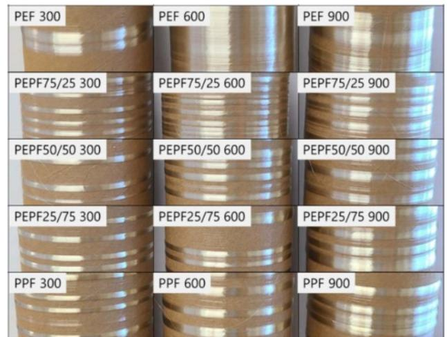
Figure 7. Melt spun copolyester fibers at winding speed of 300, 600 and 900 m/min.
