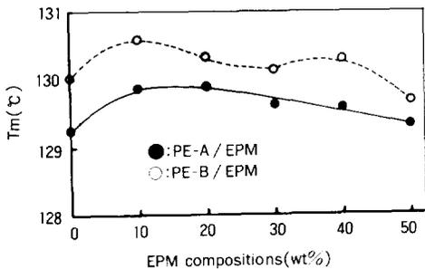
Fig. 11. Melting peak temperature( $T_m$ ) vs. composition for PE-A / EPM and PE-B / EPM blends.
