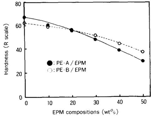
Fig. 12. Hardness vs. composition for PE-A / EPM and PE-B / EPM blends.
