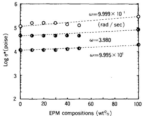
Fig. 7. Viscosity vs. composition for PE-B / EPM blends.
