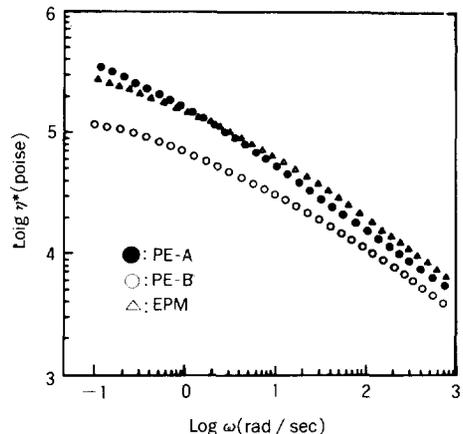
Fig. 3. Complex viscosity functions for the components.
