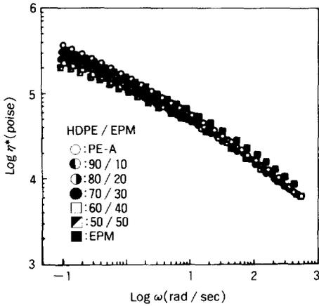
Fig. 4. Complex viscosity functions for PE-A / EPM blends.
