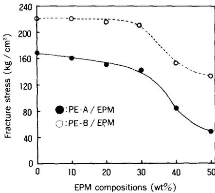
Fig. 15. Fracture stress vs. composition for PE-A / EPM and PE-B / EPM blends.
