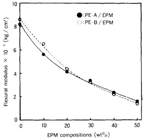
Fig. 13. Flexural modulus vs. composition for PE-A / EPM and PE-B / EPM blends.
