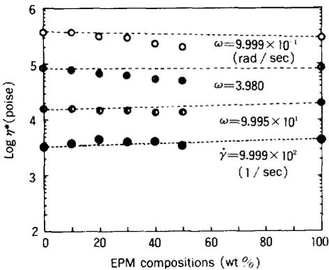
Fig. 5. Viscosity vs. composition for PE-A / EPM blends.
