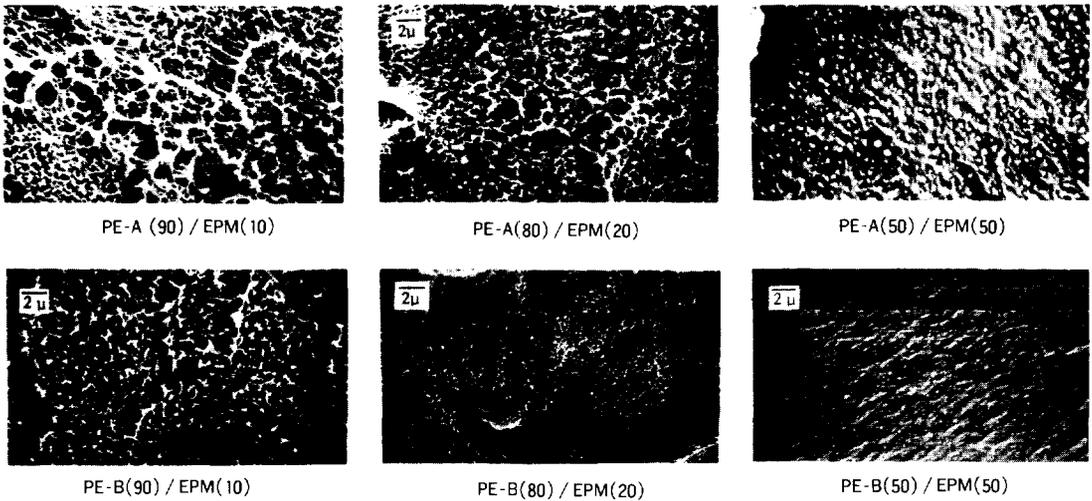
Fig. 2. Scanning electron micrographs of cryogenically fractured surfaces for PE-A / EPM and PE-B / EPM blends.
