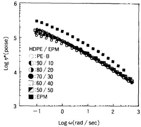
Fig. 6. Complex viscosity function for PE-B / EPM blends.
