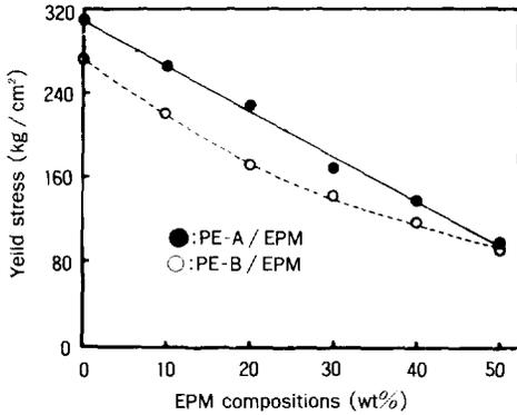
Fig. 14. Yield stress vs. composition for PE-A / EPM and PE-B / EPM blends.
