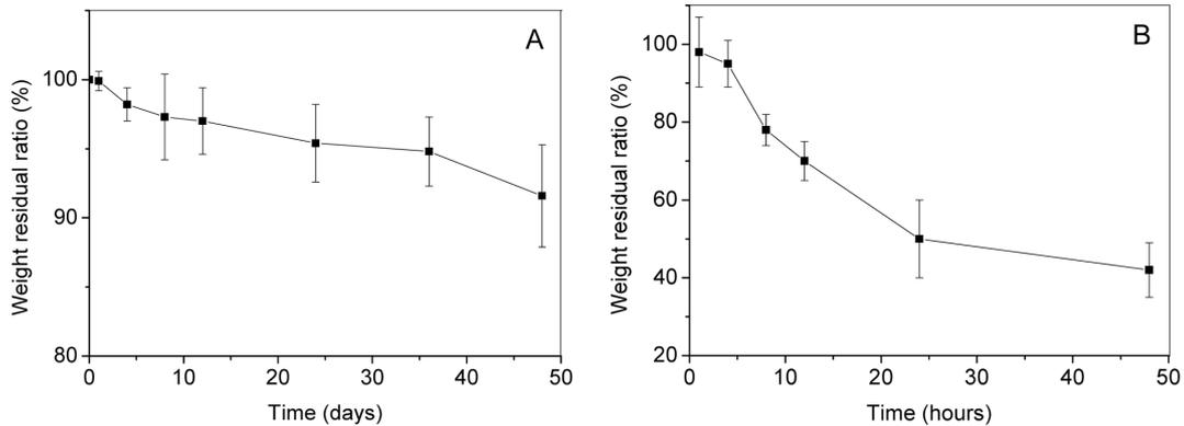
**Figure 7.** Weight of SF in degradation process in PBS solution (A); protease XIV solution (B).
