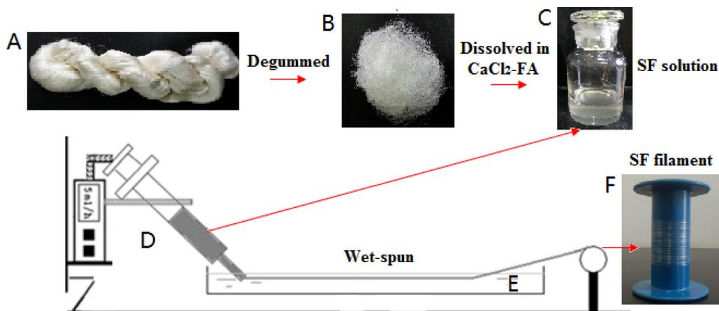
**Figure 1.** Schematic of custom-made wet-spun device for preparing SF filaments: (A) *Bombyx mori* silk; (B) degummed silk; (C) SF solution; (D) wet-spun device; (E) coagulation bath; (F) filaments.
