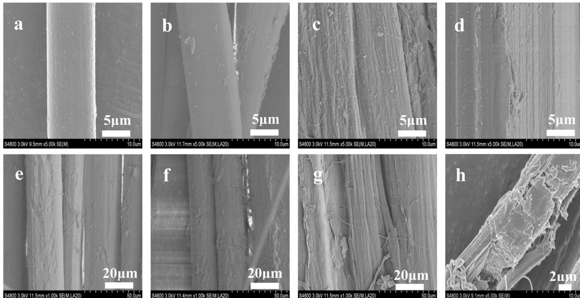
**Figure 8.** SEM of SF filament at different degradation times in PBS solution: (a) 1 d; (b) 15 d; (c) 30 d; (d) 48 d; and protease XIV solution: (e) 1 h; (f) 12 h; (g) 24 h; (h) 48 h.
