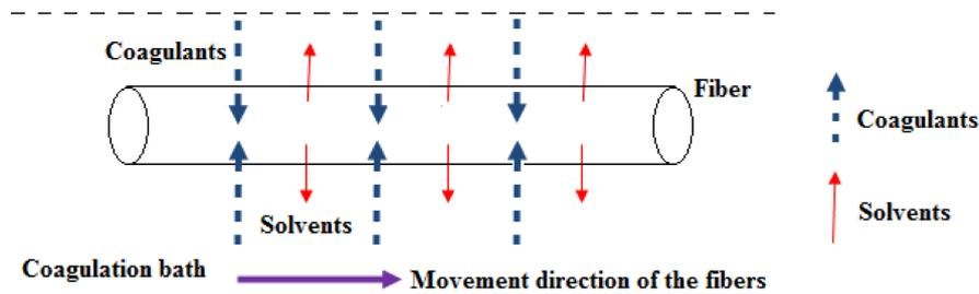
**Figure 3.** Double diffusion process in wet-spun.
