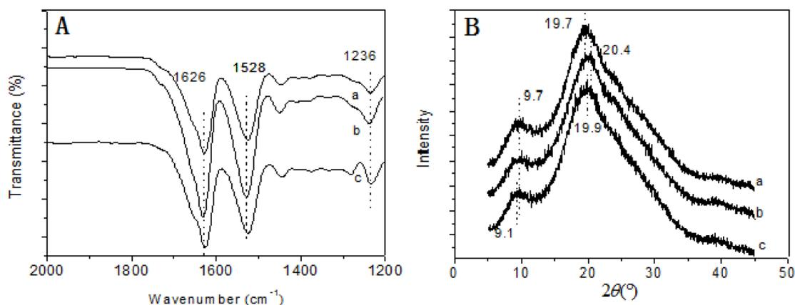
Figure 6. FTIR (A); XRD (B) results of SF filaments (a. as-spun; b. SF $\times 2$ ; c. SF $\times 3$ ).
