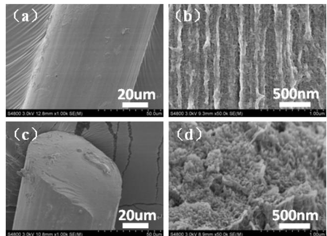
**Figure 4.** SEM images of SF filaments. Longitudinal views (a, $\times 1000$ ; b, $\times 50000$ ) and cross-section views (c, $\times 1000$ ; d, $\times 50000$ )
