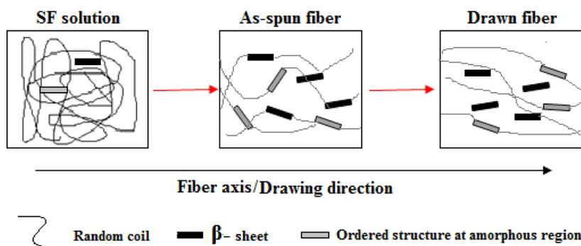
Figure 5. Schematic illustration of SF filaments structure changed in process of drawing.
