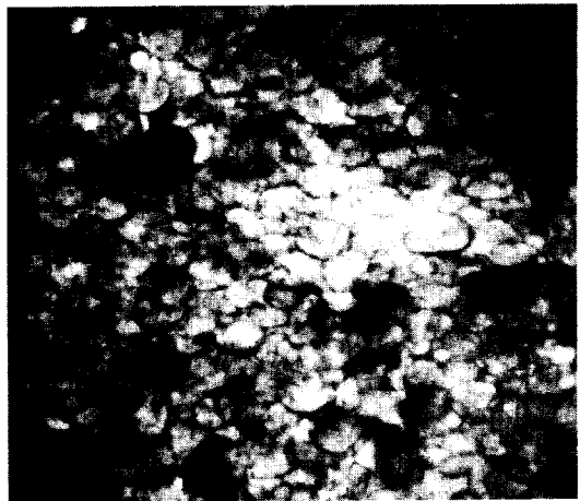
Fig. 4. The internal morphology of PCS-27 stained with \text{RuO}_4 . The dark region is PS-rich region and the bright region is PVC-rich region. (mag., \times 58,000 ).
