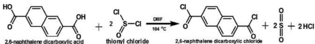
**Scheme 1.** Modification of NDA into NDC by thionyl chloride.
