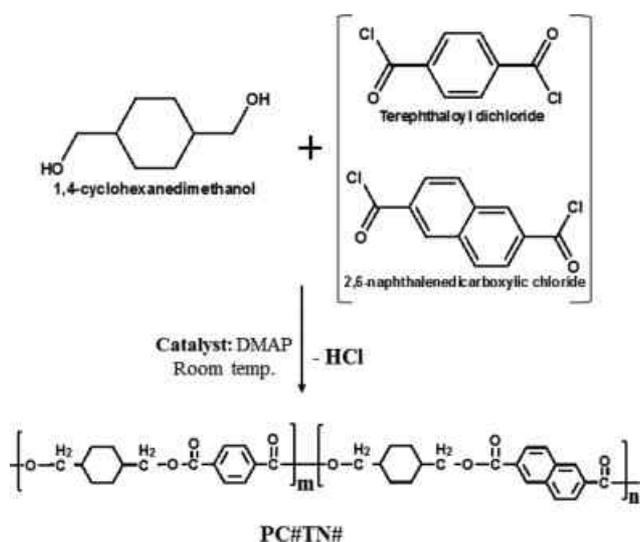
**Scheme 2.** Schematic diagram for the solution polymerization of PC#TN# series.
