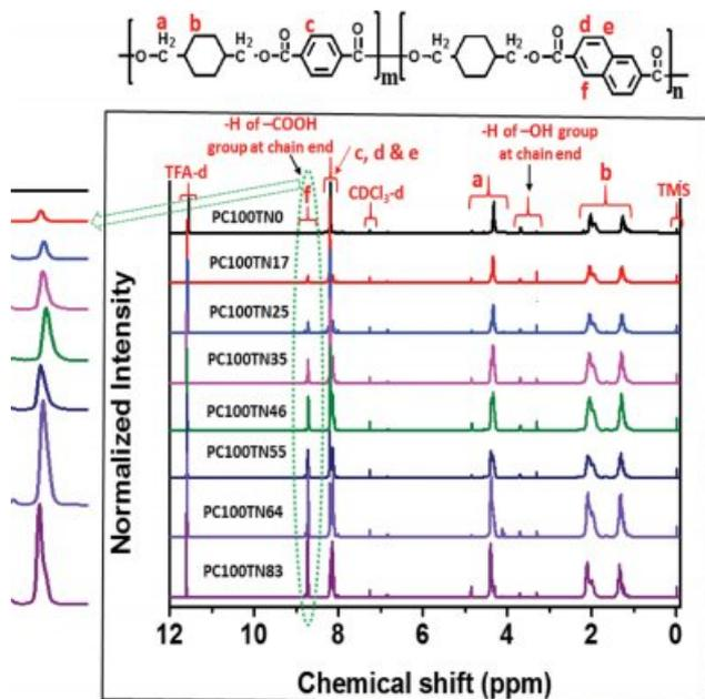
**Figure 4.**  $^1\text{H}$  NMR spectra of solution polymerized PC100TN# copolyesters with peak assignments.
