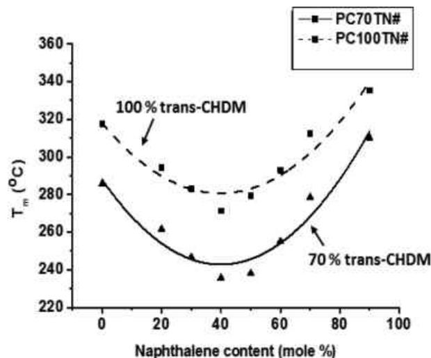
**Figure 6.** Effect of naphthalene content (mole%), defined as  $n/(m+n)$  of Scheme 1, on melting temperature ( $T_m$ ) of PC70TN# and PC100TN# copolymers.
