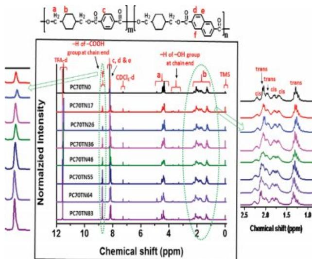
**Figure 3.**  $^1\text{H}$  NMR spectra of solution polymerized PC70TN# copolyesters with peak assignments.
