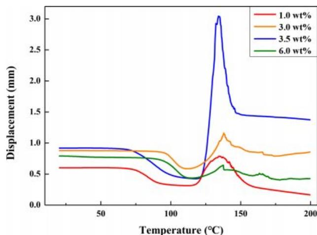
**Figure 8.** TMA thermograms of the expandable microcapsules prepared with different contents of stabilizer.
