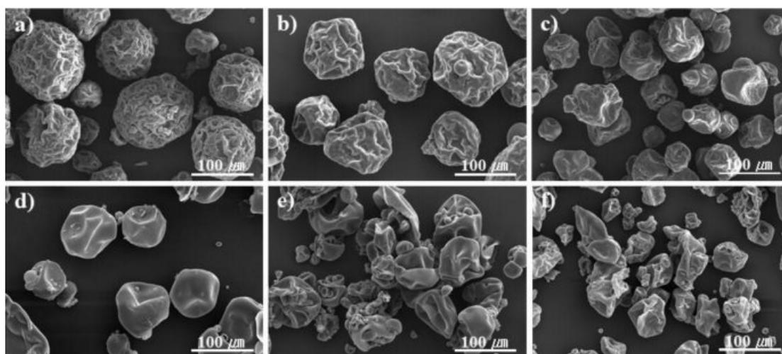
**Figure 9.** SEM microphotographs of expandable microcapsules prepared at different AN/MAN ratios: (a) 80:20; (b) 70:30; (c) 60:40; (d) 50:50; (e) 40:60; (f) 30:70 w/w.
