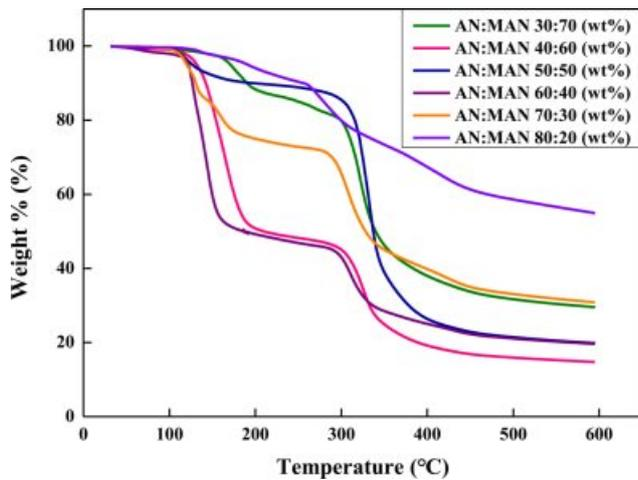
**Figure 10.** TGA thermograms of expandable microcapsules prepared at different AN/MAN ratios.
