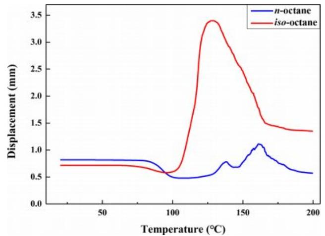
**Figure 12.** TMA thermograms of the expandable microcapsules prepared with different type of blowing agent.
