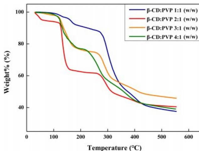
**Figure 3.** TGA thermograms of expandable microcapsules prepared at different  $\beta$ -CD/PVP ratios.
