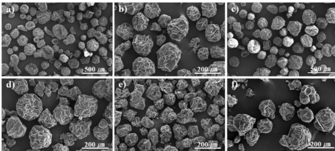
**Figure 5.** SEM microphotographs of expandable microcapsules prepared at different contents of stabilizer. (a) 1.0; (b) 3.0; (c) 3.5; (d) 6.0; (e) 9.0; (f) 12.0 wt%.
