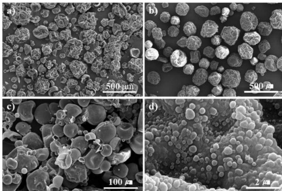
**Figure 1.** SEM microphotographs of expandable microcapsules prepared at different  $\beta$ -CD/PVP ratios: (a) 1:1; (b) 2:1; (c) 3:1; (d) 4:1 w/w.
