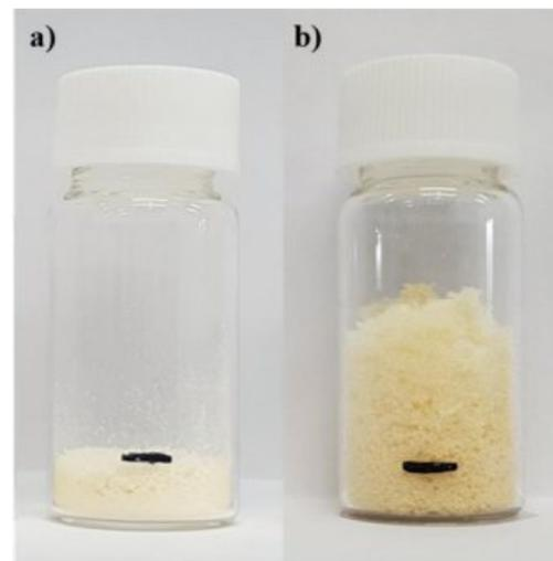
**Figure 13.** Digital photographs of (a) unexpanded microcapsules; (b) expanded microcapsules (Table 1, sample 24) at 130  $^{\circ}\text{C}$ .
