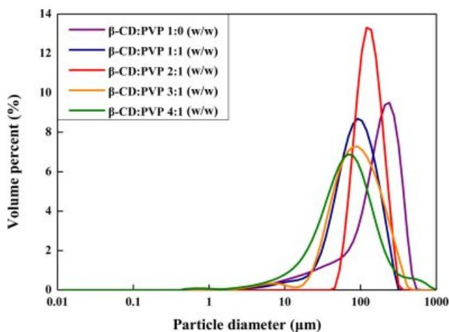
**Figure 2.** Particle size analysis of the expandable microcapsules prepared at different  $\beta$ -CD/PVP ratios.
