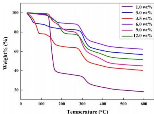
**Figure 7.** TGA thermograms of expandable microcapsules prepared with different contents of stabilizer.
