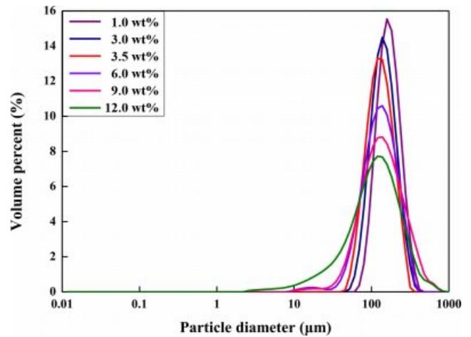
**Figure 6.** Particle size analysis of the expandable microcapsules prepared with different contents of stabilizer.
