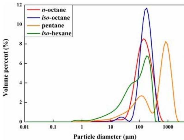
**Figure 11.** Particle size analysis of the expandable microcapsules prepared at different type of blowing agent.
