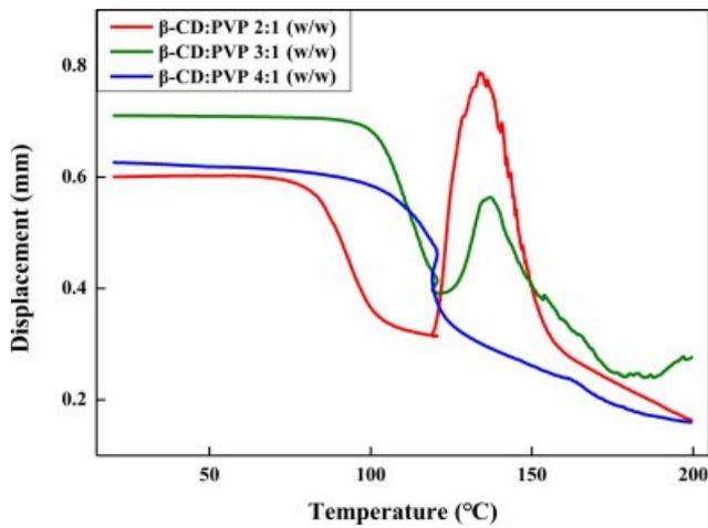
**Figure 4.** TMA thermograms of the expandable microcapsules prepared at different  $\beta$ -CD/PVP ratios.
