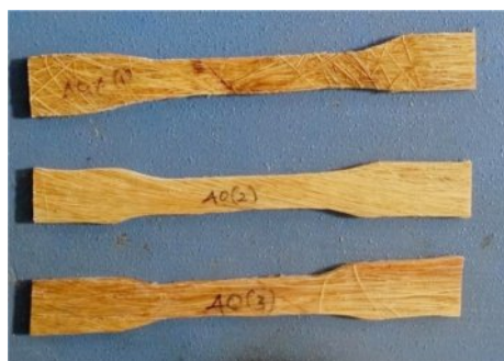
Figure 4. Peduncle fiber composite for tensile test.
