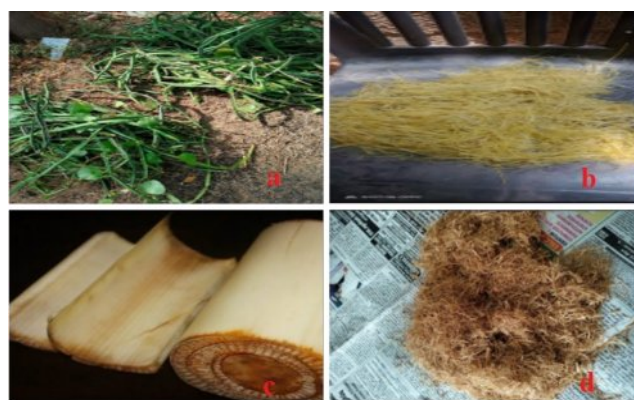
Figure 1. Fibre Extraction: (a) cissus quadrangularis stem; (b) cissus quadrangularis fiber; (c) banana stem; (d) banana fiber.
