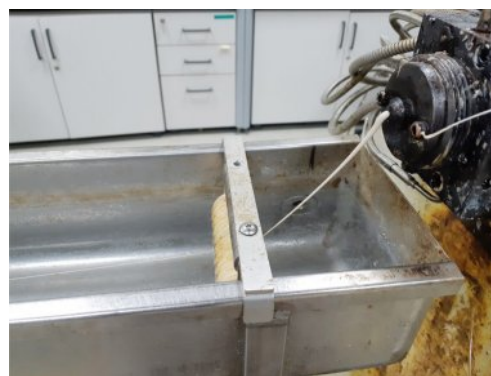
Figure 7. Photographs of the extrusion of the m-PPS/m-POE blends.
